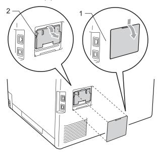
4 Unpack the SO-DIMM and hold it by its edges.
