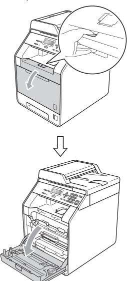
Hold the green handle of the drum unit. Pull the drum unit out until it stops.
