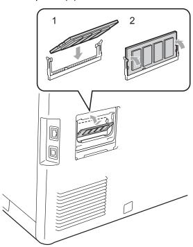
6 Put the metal (2) and then the plastic (1) SO-DIMM covers back on.
