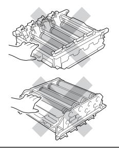
5 Hold the green handle of the belt unit with both hands and lift the belt unit up, then pull it out.
