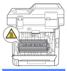
3 Pull the green tabs (2) at the left and right hand sides toward you and fold down the fuser cover (1).
