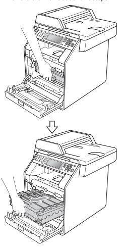
4 Hold the handle of the toner cartridge and slightly push it toward the machine to unlock it. Then pull it out of the drum unit. Repeat this for all the toner cartridges.
