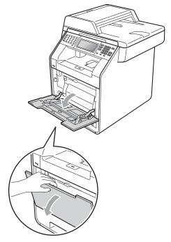
Pull out the MP tray support and unfold the flap (1).
