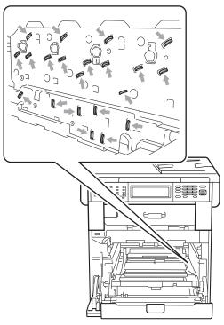
Hold the green handles of the drum unit when you carry it. DO NOT hold the sides of the drum unit.
