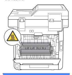
5 Push down and pull the green tabs at the left and right hand sides toward you and fold down the fuser cover (1).
