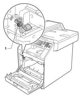
7 Match the guide ends (2) of the drum unit to the ▶ marks (1) on both sides of the machine, then gently slide the drum unit into the machine until it stops at the green lock lever.
