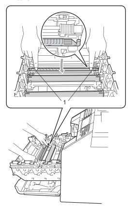
6 Clean the corona wires inside the drum unit by gently sliding the green tabs from left to right and right to left several times.
