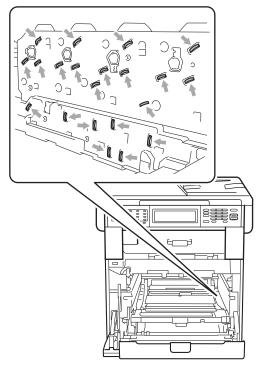
Hold the green handles of the drum unit when you carry it. DO NOT hold the sides of the drum unit. Hold the handle of the toner cartridge and slightly push it to unlock it. Then pull it out of the drum unit. Repeat this for all the toner cartridges.
