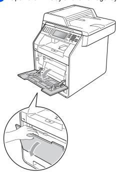
Pull out the MP tray support and unfold the flap (1).
