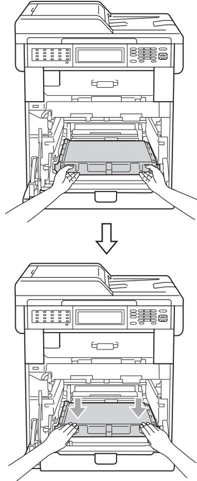
9 Install orange packing materials to the drum unit as follows:
