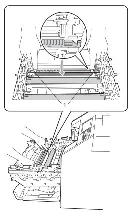
5 Clean the corona wire inside the drum unit by gently sliding the green tab from left to right and right to left several times.
