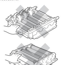
Turn the drum unit over by holding the green handles. Make sure that the drum unit gears (1) are on the left hand side.
