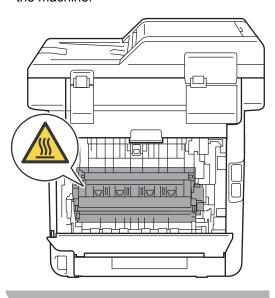
5 Push down and pull the green tabs at the left and right hand sides toward you and fold down the fuser cover (1).
