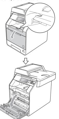
9 Hold the green handle of the drum unit. Pull the drum unit out until it stops.
