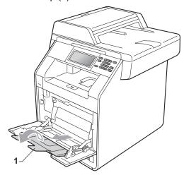
3 Lift up the support flap to prevent envelopes or sheets of thick paper from sliding off the *face-down* output tray. If the support flap is closed you should remove each envelope as soon as it comes out of the machine.
