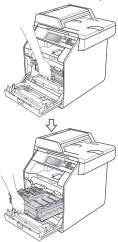
10 Turn the green lock lever (1) at the left of the machine anticlockwise to the release position. Holding the green handles of the drum unit, lift the front of the drum unit and remove it from the machine.
