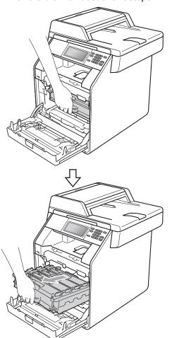
4 Hold the handle of the toner cartridge and slightly push it toward the machine to unlock it. Then pull it out of the drum unit. Repeat this for all the toner cartridges.
