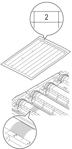
Turn the drum unit gear toward you by hand while looking at the surface of the suspected area.
