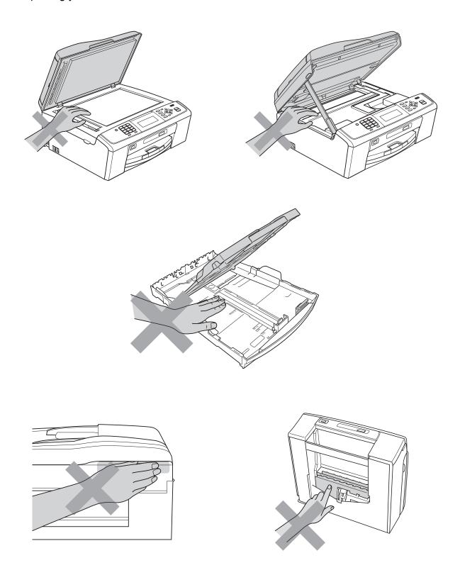
DO NOT carry the machine by holding the scanner cover or the Jam Clear Cover.
