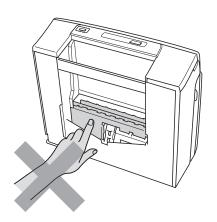
DO NOT carry the machine by holding the scanner cover or the Jam Clear Cover.
