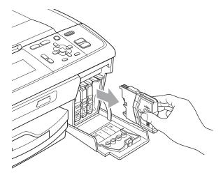
3 Open the new ink cartridge bag for the colour shown on the LCD, and then take out the ink cartridge.
