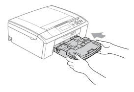
9 While holding the paper tray in place, pull out the paper support (1) until it clicks, and then unfold the paper support flap (2).
