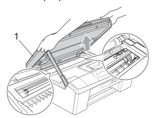
Move the print head (if necessary) to take out any paper remaining in this area. Make sure that jammed paper is not left in the corners of the machine. Check *both* ends of the print carriage.
