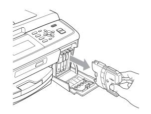
Open the new ink cartridge bag for the color shown on the LCD, and then take out the ink cartridge.
