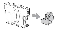
5 Each color has its own correct position. Insert the ink cartridge in the direction of the arrow on the label.
