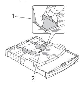
3 Put the photo paper into the photo bypass tray and gently adjust the paper side guides to the paper.
