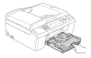
9 While holding the paper tray in place, pull out the paper support (1) until it clicks, and then unfold the paper support flap (2).
