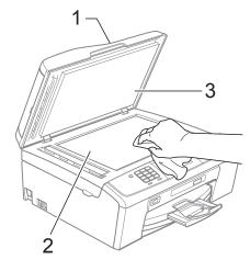
2 In the ADF unit, clean the white bar (1) and the glass strip (2) with a lint-free cloth moistened with a non-flammable glass cleaner.
