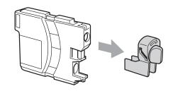
Each colour has its own correct position. Insert the ink cartridge in the direction of the arrow on the label.
