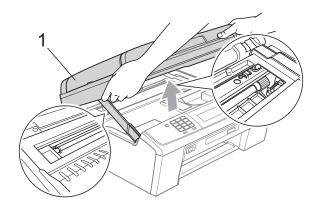
Move the print head (if necessary) to take out any paper remaining in this area. Make sure that jammed paper is not left in the corners of the machine. Check *both* ends of the print cartridge.
