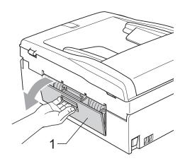
3 Clean the Paper Pick-up Rollers (1) with isopropyl alcohol on a cotton swab.
