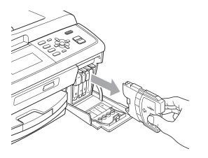
Open the new ink cartridge bag for the colour shown on the LCD, and then take out the ink cartridge.
