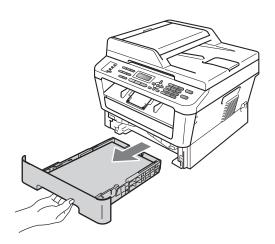
Tightly wring out a lint-free cloth soaked in lukewarm water, and then wipe the separator pad (1) of the paper tray with it to remove dust.
