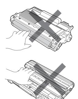
To prevent damage to the machine from static electricity, DO NOT touch the electrodes shown in the illustration.
