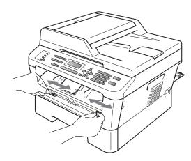
7 Using both hands, put one piece of A4 or Letter size paper in the manual feed slot until the top edge of the paper touches the paper feed roller. When you feel the machine pull in the paper, let go. The machine will start the Drum Cleaning process.
