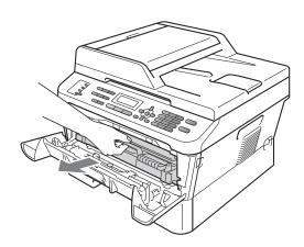
Push down the green lock lever and take the toner cartridge out of the drum unit.
