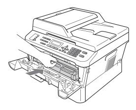
Close the front cover of the machine. If the machine does not start printing automatically, press **Start**.
