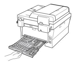
3 Pull the jammed paper out of the machine or the duplex tray.
