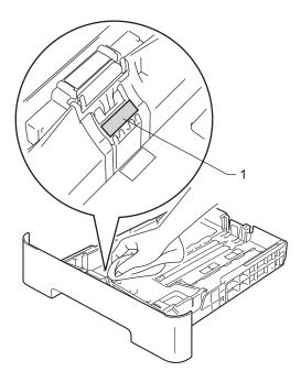
Wipe the two pick-up rollers (1) inside of the machine to remove dust.
