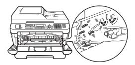
3 Clean the corona wire inside the drum unit by gently sliding the green tab from right to left and left to right several times.
