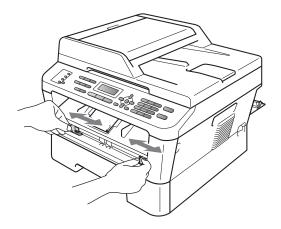
4 Using both hands, put one sheet of paper or one envelope in the manual feed slot until the front edge of the paper or envelope touches the paper feed roller. When you feel the machine pull in the paper, let go.
