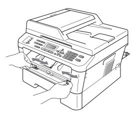
Using both hands, put one piece of A4 or Letter size paper in the manual feed slot until the top edge of the paper touches the paper feed roller. When you feel the machine pull in the paper, let go. The machine will start the Drum Cleaning process.
