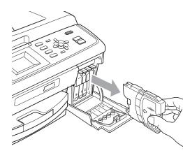
Open the new ink cartridge bag for the color shown on the LCD, and then take out the ink cartridge.
