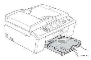
9 While holding the paper tray in place, pull out the paper support (①) until it clicks and unfold the paper support flap (②).
