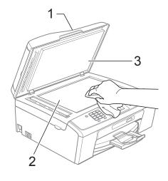
(MFC-J410 only) In the ADF unit, clean the white bar (1) and the glass strip (2) with a lint-free cloth moistened with a non-flammable glass cleaner.
