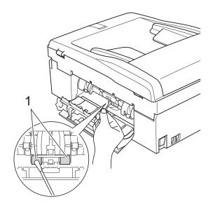
Close the Jam Clear Cover. Make sure the cover is closed correctly.
