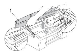
Move the print head (if necessary) to take out any paper remaining in this area. Make sure that jammed paper is not left in the corners of the machine. Check *both* ends of the print carriage.
