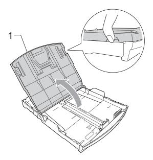
3) With both hands, gently press and slide the paper side guides (1) and then the paper length guide (2) to fit the paper size.
