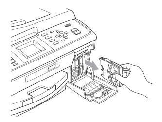
Open the new ink cartridge bag for the colour shown on the LCD, and then take out the ink cartridge.
