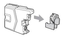
5 Each colour has its own correct position. Insert the ink cartridge in the direction of the arrow on the label.
