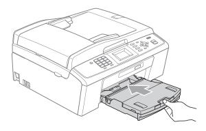
9 While holding the paper tray in place, pull out the paper support (1) until it clicks and unfold the paper support flap (2).
