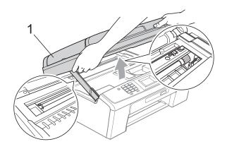
Move the print head (if necessary) to take out any paper remaining in this area. Make sure that jammed paper is not left in the corners of the machine. Check *both* ends of the print carriage.
