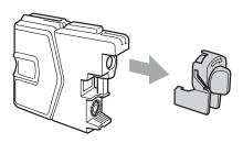
5 Each colour has its own correct position. Insert the ink cartridge in the direction of the arrow on the label.
