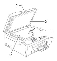
(MFC-J410 and MFC-J415W only) In the ADF unit, clean the white bar (1) and the glass strip (2) with a lint-free cloth moistened with a non-flammable glass cleaner.
