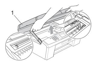
Move the print head (if necessary) to take out any paper remaining in this area. Make sure that jammed paper is not left in the corners of the machine. Check *both* ends of the print cartridge.
