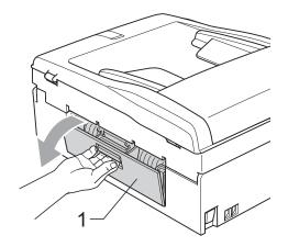
Clean the Paper Pick-up Rollers (1) with isopropyl alcohol on a cotton swab.
