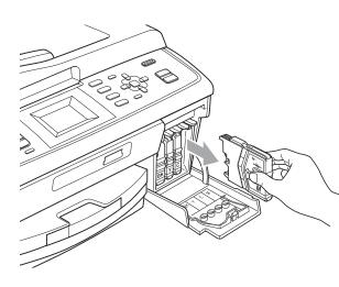
Open the new ink cartridge bag for the colour shown on the LCD, and then take out the ink cartridge.
