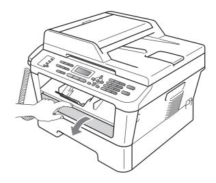
3 Using both hands, slide the manual feed slot paper guides to the width of the paper that you are going to use.
