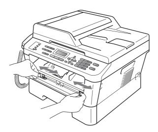
4 Using both hands, put one sheet of paper in the manual feed slot until the front edge of the paper touches the paper feed roller. When you feel the machine pull in the paper, let go.
