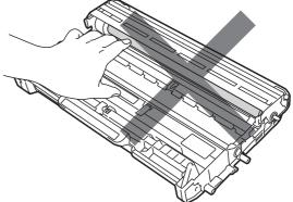
• To prevent damage to the machine from static electricity, DO NOT touch the electrodes shown in the illustration.
