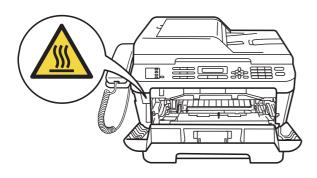
4 Push down the green lock lever and take the toner cartridge out of the drum unit.
