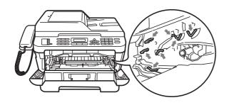
3 Push down the green lock lever and take the toner cartridge out of the drum unit.
