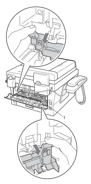
5 Using both hands, gently pull the jammed paper out of the fuser unit.
