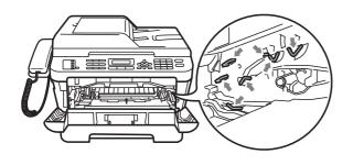
3 Clean the corona wire inside the drum unit by gently sliding the green tab from right to left and left to right several times.
