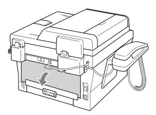
4 Pull down the tabs at the left and right hand sides to open the fuser cover (1).
