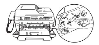
Put the print sample in front of the drum unit, and find the exact position of the poor print.
