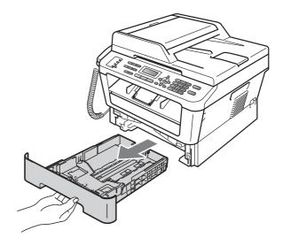
2 While pressing the green paper-guide release lever, slide the paper guides to fit the paper size you are loading in the tray. Make sure that the guides are firmly in the slots.
