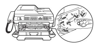
3 Push down the green lock lever and take the toner cartridge out of the drum unit. Clear the jammed paper if there is any inside the drum unit.
