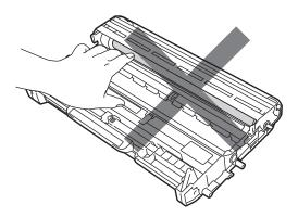
Unpack the drum unit just before you put it in the machine. Exposure to direct sunlight or room light may damage the drum unit.
