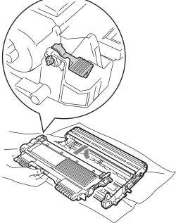
8 Clean the primary corona wire inside the drum unit by gently sliding the green tab from left to right and right to left several times.
