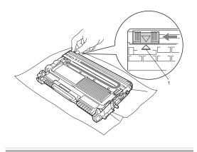
8 Put the new drum unit and toner cartridge assembly in the machine.
