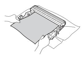
5 Turn the drum unit gear by hand while looking at the surface of the OPC drum (1).
