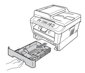
2 While pressing the green paper-guide release lever (1), slide the paper guides to fit the paper size you are loading in the tray. Make sure that the guides are firmly in the slots.
