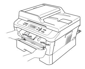
7 Using both hands, put one piece of A4 or Letter size paper in the manual feed slot until the top edge of the paper touches the paper feed roller. When you feel the machine pull in the paper, let go. The machine will start the Drum Cleaning process.
