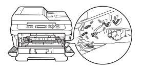
Push down the green lock lever and take the toner cartridge out of the drum unit. Clear the jammed paper if there is any inside the drum unit.
