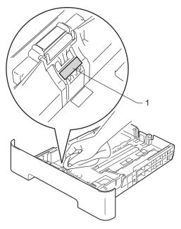
4 Wipe the two pick-up rollers (1) inside of the machine to remove dust.
