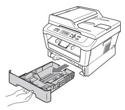
3 Tightly wring out a lint-free cloth soaked in lukewarm water, and then wipe the separator pad (1) of the paper tray with it to remove dust.
