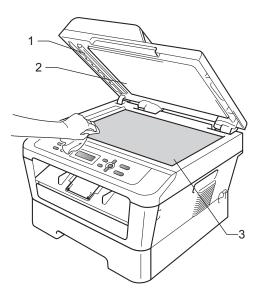
3 (For DCP-7065DN) In the ADF unit, clean the white bar (1) and the scanner glass strip (2) underneath it with a soft lint-free cloth moistened with water.
