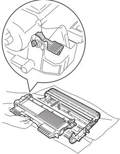
8 Put the drum unit and toner cartridge assembly back in the machine.
