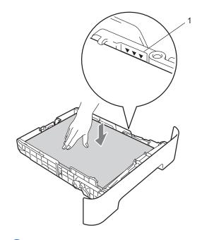
5 Put the paper tray firmly back in the machine. Make sure that it is completely inserted into the machine.
