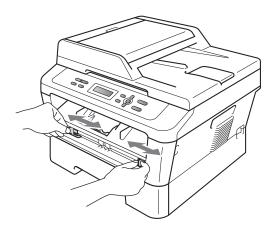
4 Using both hands, put one sheet of paper in the manual feed slot until the front edge of the paper or transparency touches the paper feed roller. When you feel the machine pull in the paper, let go.
