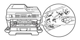
Clean the corona wire inside the drum unit by gently sliding the green tab from left to right and right to left several times.
