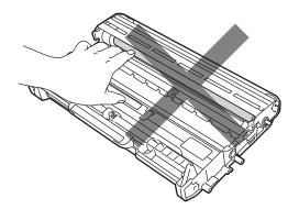
5 Put the toner cartridge back into the drum unit until you hear it lock into place. If you put the cartridge in properly, the green lock lever will lift automatically.
