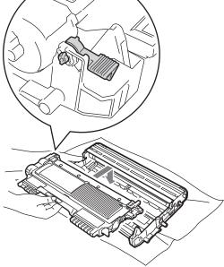
8 Clean the primary corona wire inside the drum unit by gently sliding the green tab from left to right and right to left several times.
