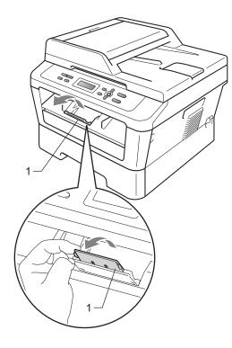
3 Using both hands, slide the manual feed slot paper guides to the width of the paper that you are going to use.
