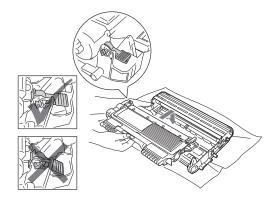
6 If you were able to remove the drum unit and toner cartridge assembly and the jammed paper, you have cleared the paper jam. Put the drum unit and toner cartridge assembly back into the machine and close the front cover. If the machine does not start printing automatically, press **Start**. Lift the scanner cover.
