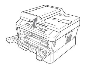
Use both hands to carefully pull the jammed paper up and out of the output tray opening.
