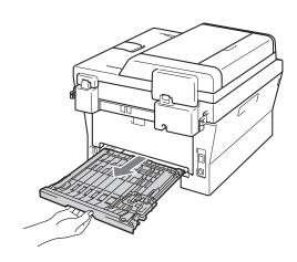
3 Pull the jammed paper out of the machine or the duplex tray.
