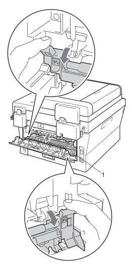
5 Using both hands, gently pull the jammed paper out of the fuser unit.
