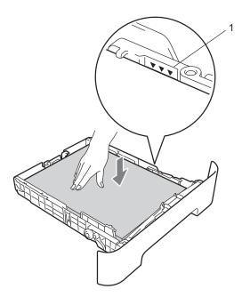
5 Put the paper tray firmly back in the machine. Make sure that it is completely inserted into the machine.
