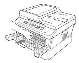
8 Close the front cover. If the machine does not start printing automatically, press **Start**.
