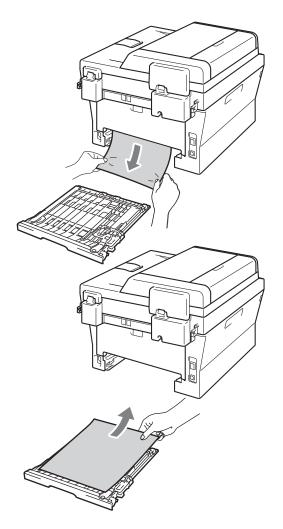
4 Make sure that the jammed paper does not remain under the machine from static electricity.
