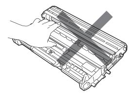
· Wait to unpack the new drum unit until immediately before you put it in the machine. Exposure to direct sunlight or room light may damage the drum unit.
