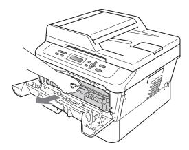
If you can not remove the drum unit and toner cartridge assembly easily, do not use extra force. Instead, go to step 7.
