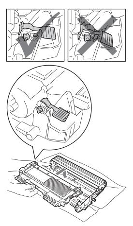
8 Clean the primary corona wire inside the drum unit by gently sliding the green tab from left to right and right to left several times.
