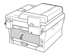
Pull down the tabs at the left and right hand sides to open the fuser cover (1).
