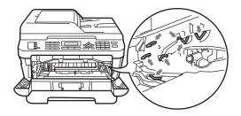
3 Clean the corona wire inside the drum unit by gently sliding the green tab from left to right and right to left several times.
