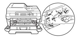
4 Push down the green lock lever and take the toner cartridge out of the drum unit. Clear the jammed paper if there is any inside the drum unit.
