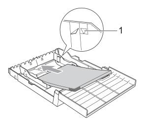
6 Using both hands, gently adjust the paper side guides so they touch the sides of the paper stack.
