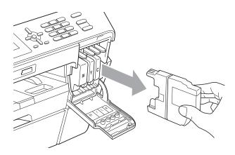
3 Open the new ink cartridge bag for the color shown on the LCD, and then take out the ink cartridge.
