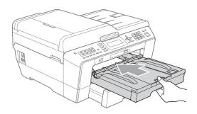
13 Pull out the paper support (1) until it clicks and unfold the paper support flap (2).
