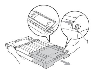
Open the output paper tray cover and adjust the paper length guide (1) for the paper.
