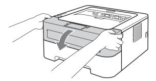
2 Slowly take out the drum unit and toner cartridge assembly. The jammed paper may be pulled out with the drum unit and toner cartridge assembly, or this may release the paper so you can pull it out from inside of the machine.
