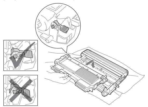
8 Clean the primary corona wire inside the drum unit by gently sliding the green tab from right to left and left to right several times.
