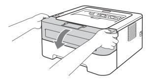
2 Slowly take out the drum unit and toner cartridge assembly. The jammed paper may be pulled out with the drum unit and toner cartridge assembly, or this may release the paper so you can pull it out of the inside of the machine.
