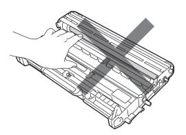
5 Put the print sample in front of the drum unit, and find the exact position of the poor print.
