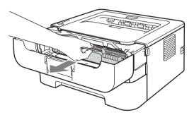
4 Push down the green lock lever and take the toner cartridge out of the drum unit.
