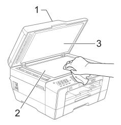
In the ADF unit, clean the white bar (1) and the glass strip (2) with a soft lint-free cloth moistened with a non-flammable glass cleaner.
