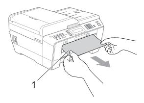
4 Lift the Jam Clear flap, and remove the jammed paper.
