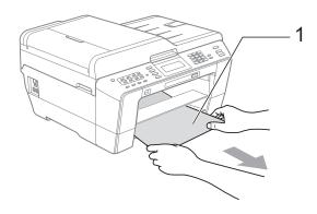
4 Lift the flap, and remove the jammed paper.
