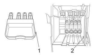
If you are not able to find the orange protective part, DO NOT remove the ink cartridges before shipping. It is essential that the machine be shipped with either the orange protective part or the ink cartridges in position. Shipping without them will cause damage to your machine and may void your warranty. When travelling with the ink cartridges still in the machine please keep the machine upright as this will protect the machine from leakage. 9 Wrap the machine in the bag.
