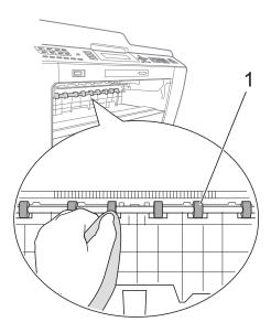
3 Lift the Jam Clear flap (2), and then clean the back side of the Paper Feed Rollers (1) with a soft lint-free cloth moistened with water.
