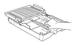
5 Close the output paper tray cover and put the output paper tray firmly back in the machine.
