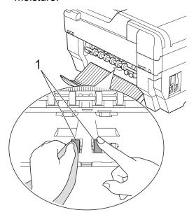
Olean the Back Paper Feed Rollers (1) with a soft lint-free cloth moistened with water.
