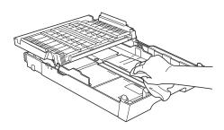
Close the output paper tray cover and put the output paper tray firmly back in the machine.
