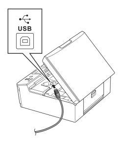
C Carefully guide the USB cable into the cable channel and out the back of the machine. Connect the cable to your computer.
