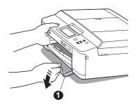
Remove the plastic bag 2 containing the ink cartridges from on top of the paper tray.
