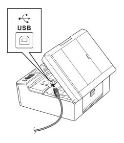
Carefully guide the USB cable into the cable channel and out the back of the machine. Connect the cable to your computer.
