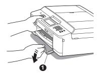
Remove the plastic bag ② containing the ink cartridges from on top of the paper tray.
