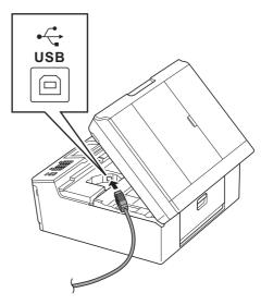
Carefully guide the USB cable into the cable channel and out the back of the machine.
