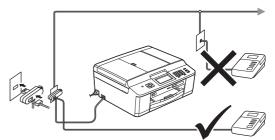
Set the receive mode to External TAD if you have an external answering machine. See Choose a Receive Mode on page 7. (Detailed information ➤> Basic User's Guide: Connecting an external TAD (telephone answering device))
