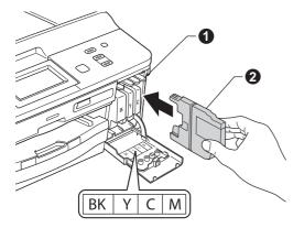
Gently push the back of the ink cartridge marked "PUSH" until it clicks. After all the ink cartridges are installed close the ink cartridge cover.
