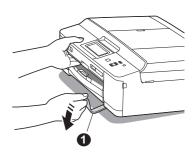
Remove the plastic bag 2 containing the ink cartridges from on top of the paper tray.
