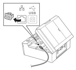
Carefully guide the network cable into the cable channel and out the back of the machine. Connect the cable to your network.
