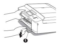
Remove the plastic bag ② containing the ink cartridges from on top of the paper tray.
