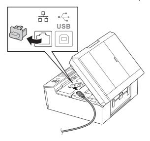
Carefully guide the network cable into the cable channel and out the back of the machine.
