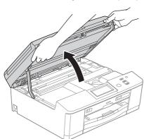
You will find the Ethernet port marked with a symbol inside the machine on the left as shown below. Remove the protective cap and connect the network cable to the Ethernet port.
