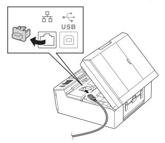
Carefully guide the network cable into the cable channel and out the back of the machine. Connect the cable to your network.
