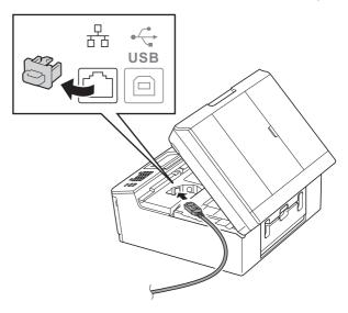
Carefully guide the network cable into the cable channel and out the back of the machine.
