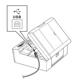
C Carefully guide the USB cable into the cable channel and out the back of the machine. Connect the cable to your Macintosh.
