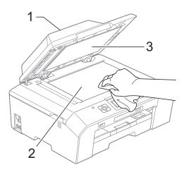
3 In the ADF unit, clean the white bar (1) and the glass strip (2) with a lint-free cloth moistened with a non-flammable glass cleaner.
