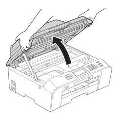
Lift the scanner cover (1) to release the lock. Gently push the scanner cover support down (2) and close the scanner cover (3) using both hands. The paper you inserted will be fed through the machine and ejected.
