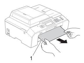
4 Lift the Flap, and remove the jammed paper.
