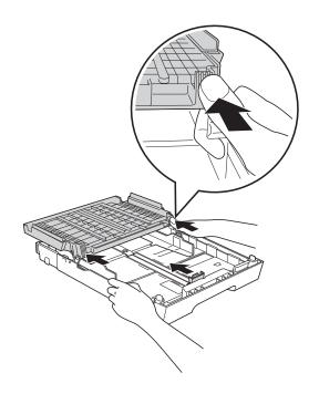
6 Gently adjust the paper side guides (1) to the paper using both hands. Make sure the paper side guides touch the sides of the paper.
