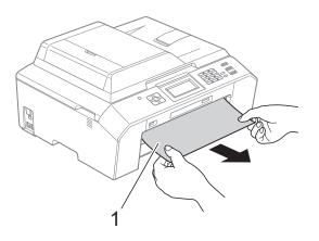
4 Lift the Jam Clear Flap, and remove the jammed paper.
