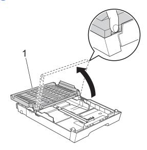
3 With both hands, gently press and slide the paper length guide (1) and then the paper side guides (2) to fit the paper size.
