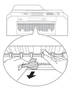
5 Open the Jam Clear Cover (1) at the back of the machine.
