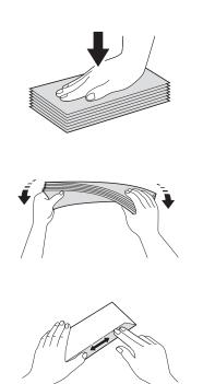
2 Put envelopes or postcards in the paper tray with the address side down. If the envelope flaps are on the long edge, load the envelopes with the flap on the left, as shown in the illustration. Load postcards with the leading edge in first. Using both hands, gently press and slide the paper length guide (1) and paper side guides (2) to fit the size of the envelopes or postcards.
