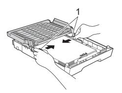
Close the output paper tray cover. Check that the paper is flat in the tray and below the maximum paper mark (1).
