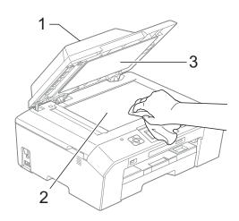
In the ADF unit, clean the white bar (1) and the glass strip (2) with a lint-free cloth moistened with a non-flammable glass cleaner.
