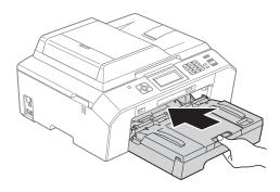
While holding the paper tray in place, pull out the paper support (1) until it clicks and unfold the paper support flap (2).
