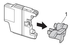
Each color has its own correct position. Insert the ink cartridge in the direction of the arrow on the label.
