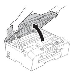
Lift the scanner cover (1) to release the lock. Gently push the scanner cover support down (2) and close the scanner cover (3) using both hands. The paper you inserted will be fed through the machine and ejected onto the output paper tray cover.
