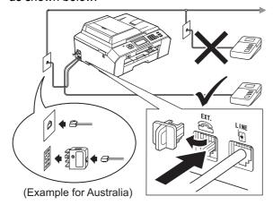
Set the receive mode to External TAD if you have an external answering machine. See Choose a Receive Mode on page 8. Detailed information >>Basic User's Guide: Connecting an external TAD (telephone answering device)
