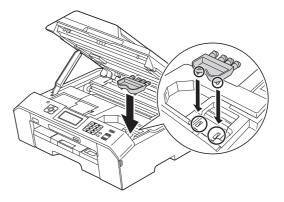
Lift the scanner cover to release the lock 1.
