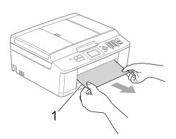
5 Lift the Jam Clear Flap, and remove the jammed paper.
