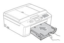
9 While holding the paper tray in place, pull out the paper support (1) until it clicks, and then unfold the paper support flap (2).
