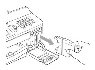
3 Open the new ink cartridge bag for the colour shown on the LCD, and then take out the ink cartridge.
