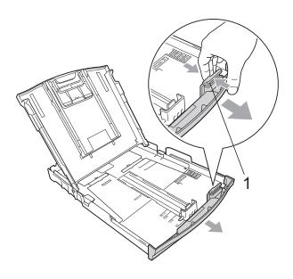
Fan the stack of paper well to avoid paper jams and misfeeds.
