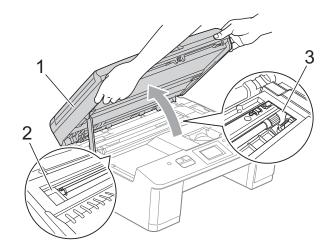
Move the print head (if necessary) to take out any paper remaining in this area. Make sure that jammed paper is not left in the corners of the machine (2) and (3).
