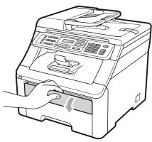
3 Using both hands, slide the manual feed slot paper guides to the width of the paper that you are going to use.
