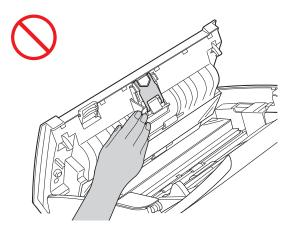
DO NOT carry the machine by holding the top cover. Doing this may cause the machine to slip out of your hands. Only carry the machine by placing your hands under the entire machine.
