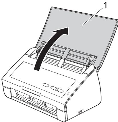
**c** Pull the Output Tray out of the machine and then unfold the Document Stopper.
