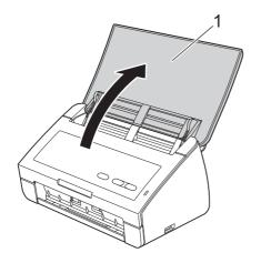
Pull the Output Tray out of the machine and then unfold the Document Stopper.
