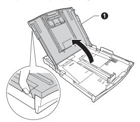
C With both hands, gently press and slide the paper side guides ● and then the paper length guide ② to fit the paper size.
