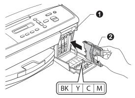
Gently push the ink cartridge until it clicks. After all the ink cartridges are installed close the ink cartridge cover.
