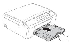
While holding the paper tray in place, pull out the paper support ① until it clicks, and then unfold the paper support flap ②.
