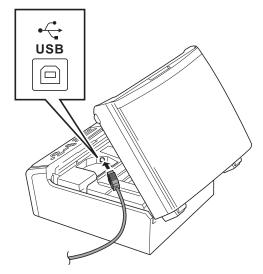
C Carefully guide the USB cable into the cable channel and out the back of the machine. Connect the cable to your Macintosh.
