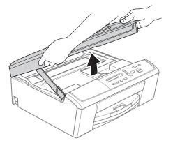
Connect the USB cable to the USB port marked with a 🚭 symbol. You will find the USB port inside the machine as shown below.
