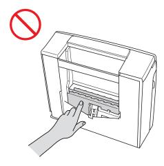
DO NOT carry the machine by holding the scanner cover or the Jam Clear Cover. Doing this may cause the machine to slip out of your hands. Only carry the machine by placing your hands under the entire machine.
