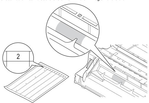
11 Turn the drum unit gear toward you by hand while looking at surface of the suspected area.
