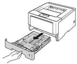
While pressing the green paper-guide release lever (1), slide the paper guides to fit the paper you are loading in the tray. Make sure that the guides are firmly in the slots.
