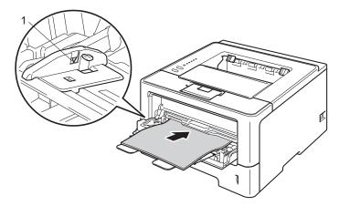
4 Lift up the support flap to prevent paper from sliding off the face-down output tray, or remove each page as soon as it comes out of the machine.
