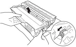
9 Turn the drum unit as shown in the illustration. Make sure that the drum unit gear (1) is on the left hand side.
