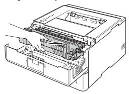
8 When you *replace* the drum unit with a new one, you need to reset the drum counter. To do this, press and hold down the **Go** for about 4 seconds until all the LEDs light up. Once all six LEDs are lit, release **Go**.
