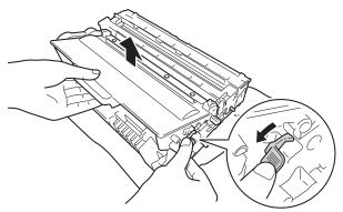
9 Put the toner cartridge back into the drum unit until you hear it lock into place. If you put the cartridge in correctly, the green lock lever on the drum unit will lift automatically.
