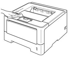
4 Pull the paper tray completely out of the machine.
