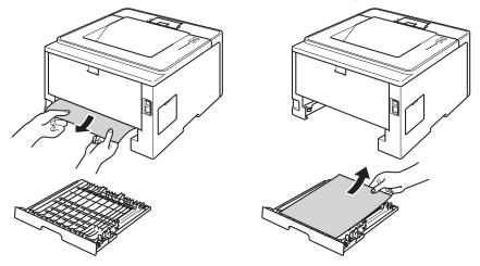
13 Make sure that the jammed paper does not remain under the machine from static electricity.
