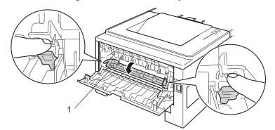
8 Using both hands, gently pull the jammed paper out of the fuser unit.
