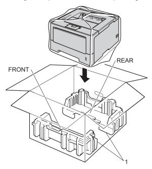
5 Put the packing material (2) marked "FRONT" on the front of the machine. Put the packing material (3) marked "REAR" on the back of the machine.
