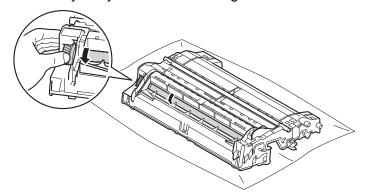
When you have found the mark on the drum that matches the drum dot check sheet, wipe the surface of the drum gently with a cotton swab until the mark on the surface comes off.
