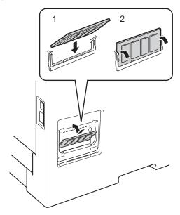
6 Put the metal (2) and then the plastic (1) SO-DIMM covers back on.
