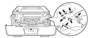
4 Clean the corona wire inside the drum unit by gently sliding the green tab from left to right and right to left several times.
