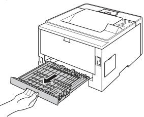
Pull the jammed paper out of the machine or out of the duplex tray.
