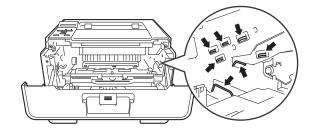
Clean the corona wire inside the drum unit by gently sliding the green tab from left to right and right to left several times.
