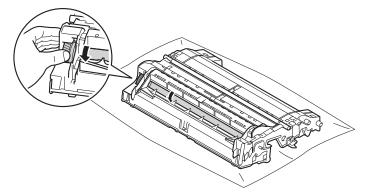
(12) When you have found the mark on the drum that matches the drum dot check sheet, wipe the surface of the drum gently with a cotton swab until the mark on the surface comes off.
