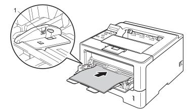
4 Lift up the support flap to prevent paper from sliding off the face-down output tray, or remove each page as soon as it comes out of the machine.
