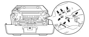
4 Push down the green lock lever and take the toner cartridge out of the drum unit.
