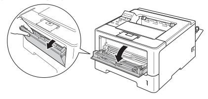
3 Pull out the MP tray support (1) and unfold the flap (2).
