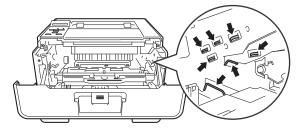
8 Push down the green lock lever and take the toner cartridge out of the drum unit.
