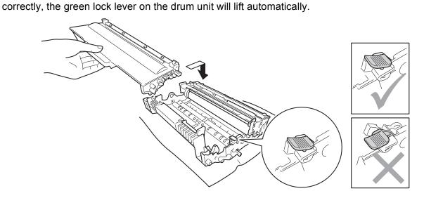
Put the new toner cartridge firmly into the drum unit until you hear it lock into place. If you put it in
