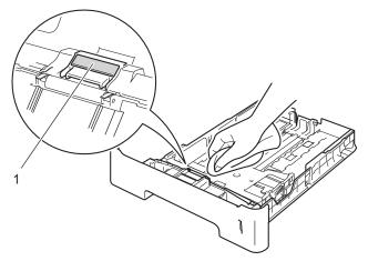
5 Wipe the two pick-up rollers (1) inside of the machine to remove dust.
