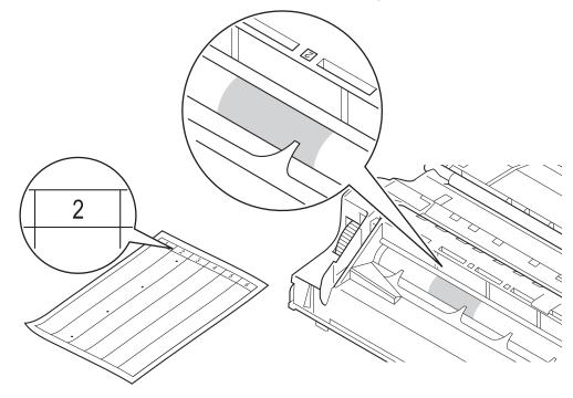
1 Turn the drum unit gear toward you by hand while looking at surface of the suspected area.
