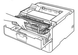
8 When you *replace* the drum unit with a new one, you need to reset the drum counter. Hold down **Go** until the Drum Clear message is displayed on the LCD, then release **Go**.
