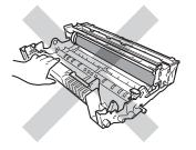
• We recommend that you place the toner cartridge on a clean, flat, level, stable surface with a sheet of disposable paper or cloth underneath it in case you accidentally spill or scatter toner.
