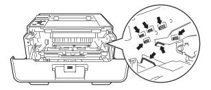
4 Push down the green lock lever and take the toner cartridge out of the drum unit.
