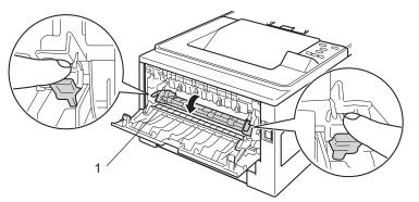
6 Using both hands, gently pull the jammed paper out of the fuser unit.
