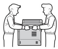
If you use a Lower Tray, DO NOT carry the machine with the Lower Tray as you may be injured or cause damage to the machine because it is not attached to the Lower Tray.
