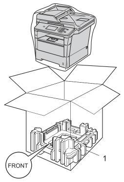
Dut the packing material (2) marked "RIGHT" on the right of the machine. Put the packing material (3) marked "LEFT" on the left of the machine. Put the AC power cord and printed materials in the original carton as shown in the illustration.
