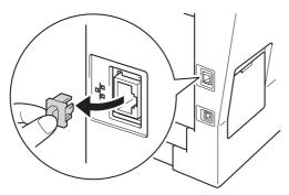
C Connect the network interface cable to the Ethernet port and then connect it to a free port on your hub.
