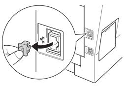
Connect the network interface cable to the Ethernet port and then connect it to a free port on your hub.
