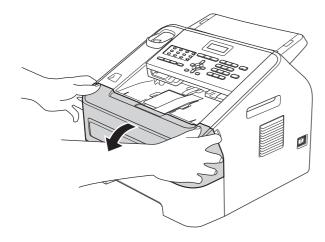
Remove the Silica Pack from the inside of the machine.
