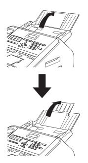
Open the control panel cover by lifting it toward the back.
