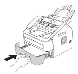
Unfold the support flap • to prevent paper from sliding off the face-down output tray.
